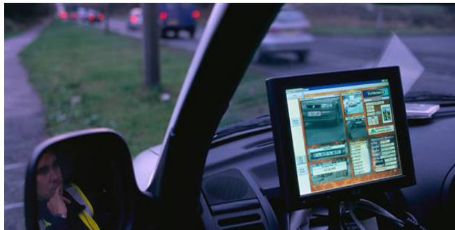
Figure 8 - An ALPR system monitors the roads of Manchester, England, checking motorists identity compared to three databases. Photo courtesy of MSNBC. http://www.msnbc.msn.com/id/15221111/
